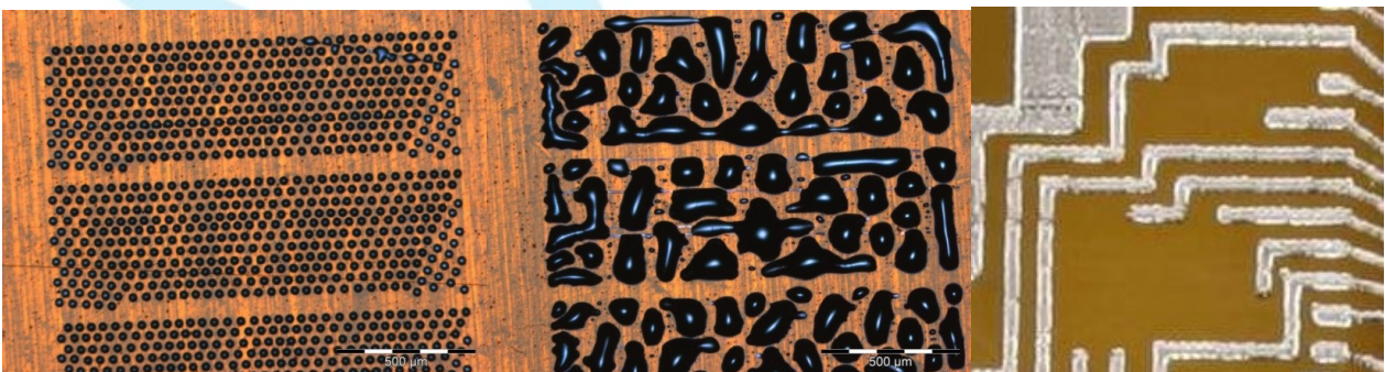
Figure 1. Left: A printing result with low resolution. Middle: A printing result in medium resolution with bulging phenomenon. Right: Result with high resolution DropFoil™.
